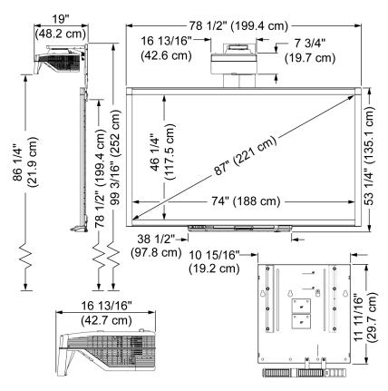
SMART Board 885ix2 interactive whiteboard Weight 60 lb. (27.2 kg) Shipping dimensions 4 3/8" W × 56 3/4" H × 88" D (11.1 cm × 144.1 cm × 223.5 cm) Shipping weight SB885ix2 90 lb. (40.8 kg) Shipping weight SB885ix2-SMP
