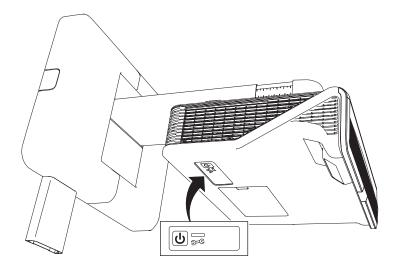
• The ECP's **Power** U button (see *Using the Extended Control Panel (ECP)* on page 27) also functions as a status light.
