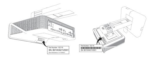
The ECP has its own serial number, which is different from the interactive whiteboard serial number. The ECP serial number is located on the bottom of the ECP.
