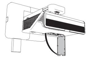
5. Use a Phillips screwdriver to loosen the two captive screws from the bottom of the lamp module.
