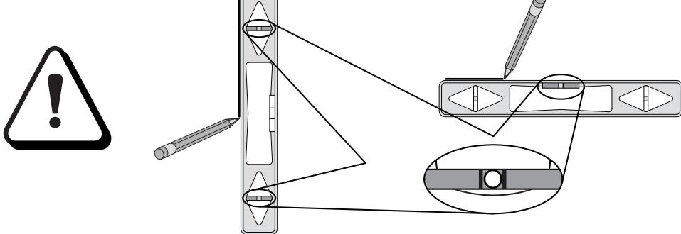
All of the lines that you draw to install the SB800i6/SB800i6-SMP must be straight and level on a plumb wall. You must install the unit straight, level and plumb for it to operate properly.
